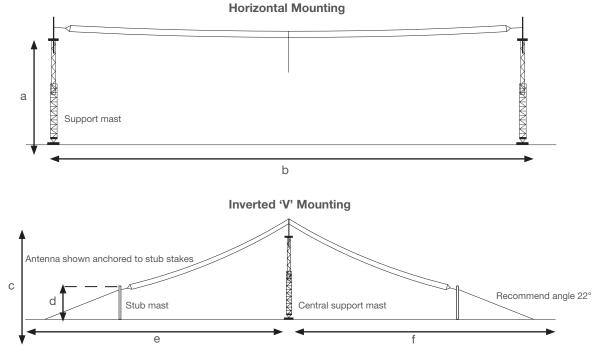
Note: Antenna should be orientated at right angles to the preferred direction of propagation to maximise network performance.
